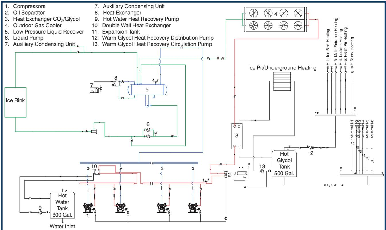
**Figure 1:** Schematic of CO<sub>2</sub> refrigeration system that does not use any secondary fluid to cool the concrete slab.
