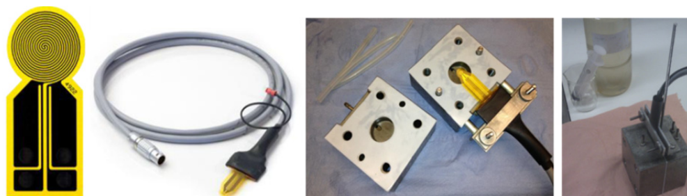
Figure 48: The Hot Disk ® Kapton sensor (left) and the sample holder with the sandwiched sensor (right)
