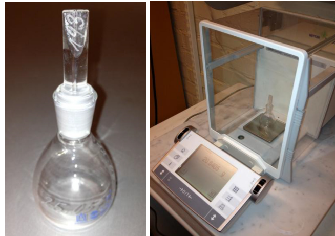
Figure 50: The pycnometer (left) and the Mattler Toledo weighing scale (right)
