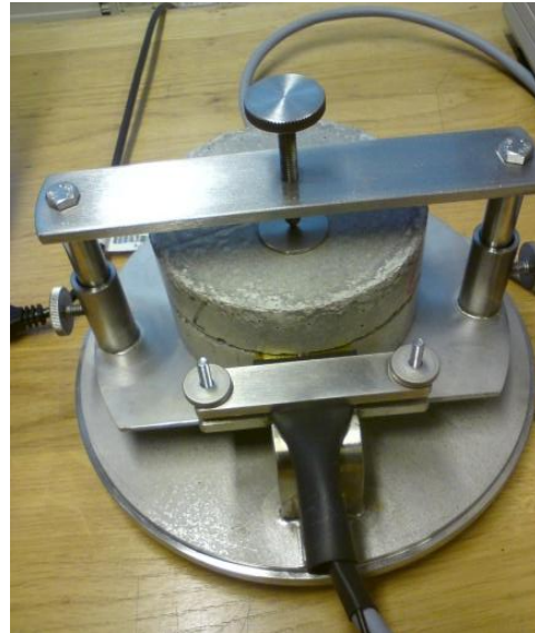
b) Assembling the sensor in the room-temperature - the solid sample holder
